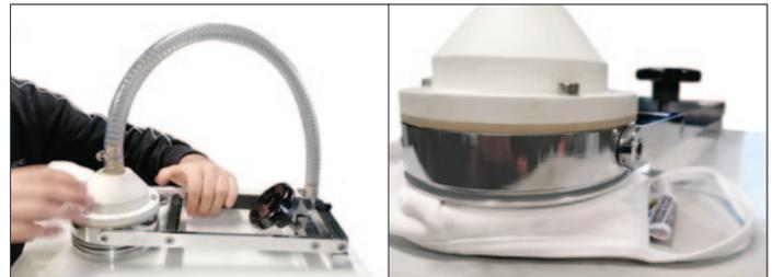
Mesdan developed a “Medical mask testing kit” according to EN 14683:2019 (Annex C) and ASTM F2100:2019 (point 9.2), for what refers to the differential pressure only, measuring the pressure difference above and below the specimen, used mainly for surgical masks.
