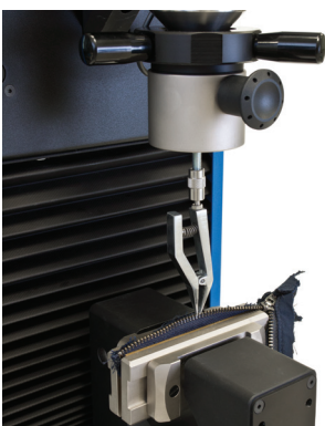
Element for Zipper Kit ( Code 194E.28 ), in compliance with ASTM D2061 Standard
