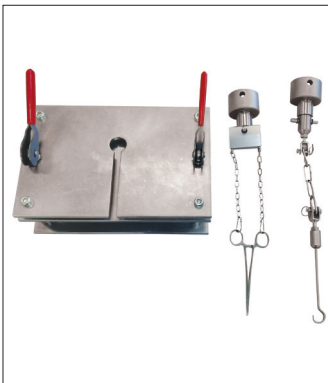
Special Testing Kit, according to ISO 4919 Tuft withdrawal force. Available on demand.
