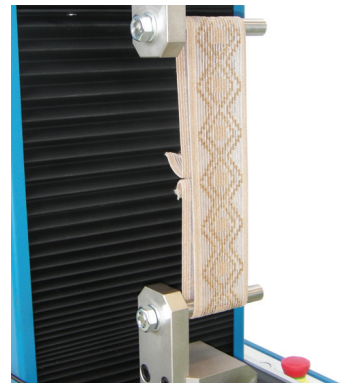
Mechanical Loop Clamps for stretch & recovery evaluation, according to ASTM D4964, Code 2510.932
