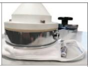
Mesdan developed a "Medical mask testing kit" according to EN 14683:2019 (Annex C) and ASTM F2100:2019 (point 9.2), for what refers to the differential pressure only, measuring the pressure difference above and below the specimen, used mainly for surgical masks.
