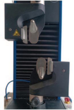
Pneumatic Clamps ("Bollard") for high-tenacity yarns, Code 2512E.760 *
