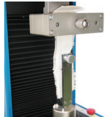
Nail tearing tool, bottom part (UNI 7275), Code 2512A.856
