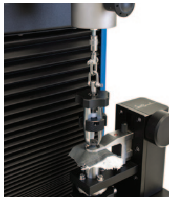
Upper Universal Grip ( Code 2510.151 ), Lower Fabric Clamp ( Code 2510.150 ), for buttons, etc.
