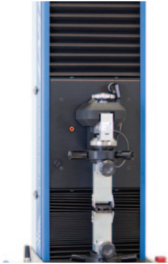
Fibre bundle 0" & 1/8" Clamps (Pressley Method), Code 331A.2 (clamps) + Code 331A.8 (clamps holders) *
