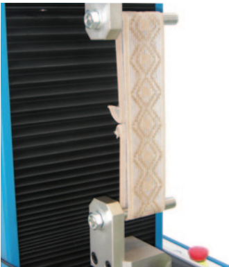
Mechanical Loop Clamps for stretch & recovery evaluation, according to ASTM D4964, Code 2510.932
