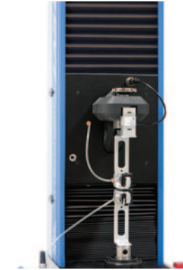
Pneumatic Clamps for single fibre, ( Code 2512E.725 ) *
