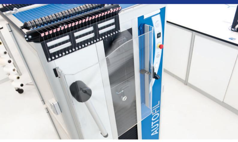
Fully automatic 24-position yarn strength tester. It can test hanks and fabrics as well in the semi-automatic mode.
