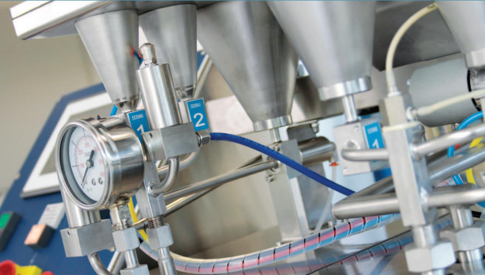
Miniature Laboratory PILOT piece dyeing machine, replicates Bulk Dyeing and fills the void between regular IR Lab dyeing machine and bulk production machine.
