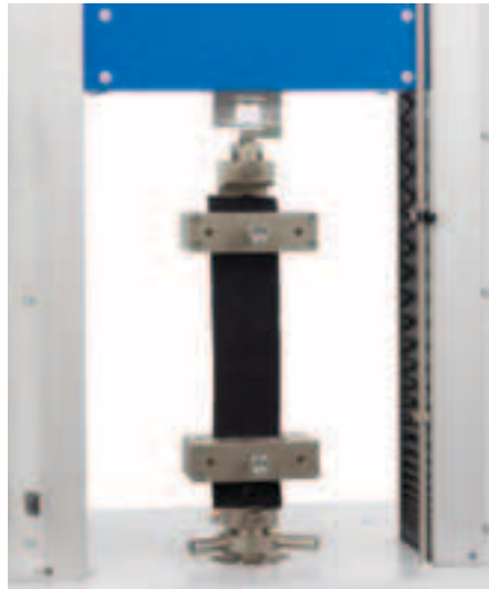
Mechanical clamps with rubber jaws, 100mm wide, Code 2510.846
