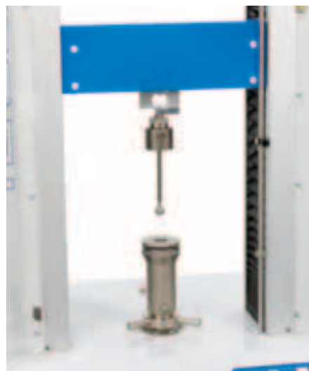
Tool for perforation test of non-wovens, Persoz type, Code 2510.800
