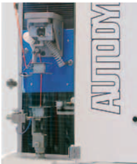
Mini clamps for yarns up to 20N (for Autodyn only), Code 2513.918 . Maxi clamps for yarns up to 50N (for Autodyn only), Code 2513.930
