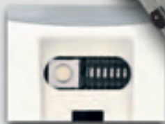
fig. 3: DIP switches for operator settings, such as update rates, memory mode, etc.
