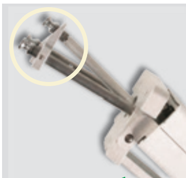
fig. 2: Filament guide for easy material acquisition of running filaments;
