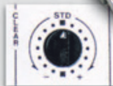
fig. 1: Field adjustment function for fine tuning of the calibration for materials which differ from factory standard calibration material; the displayed value can be increased or decreased in \pm 1.5\% increments
