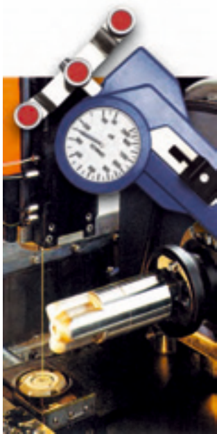
In the Wire EDM Industry The correct adjusted tension is the condition for best exact cuts
