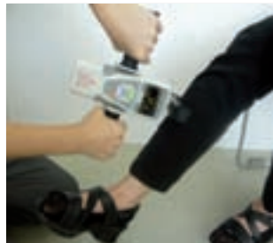
Measuring the leg muscle strength with the curved pad
