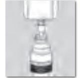
Contact point test: Measurement of contact point operating force.
