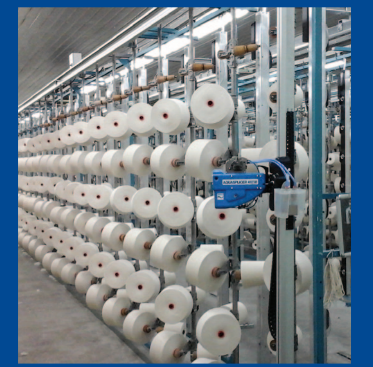
ATS "L" type with AQUASPLICER® 4923B on a sliding bar with swivel joint enabling splicer vertical movement on the Ball Warping creel .
