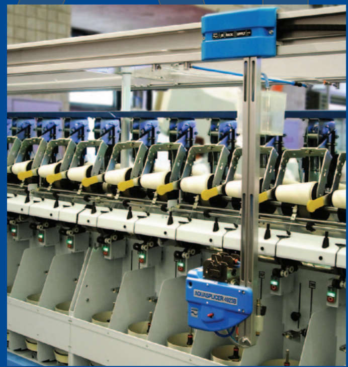
ATS "L" type fitting AQUASPLICER® 4923B installed on two-for-one twisting machine processing fine plied compact cotton yarn.
