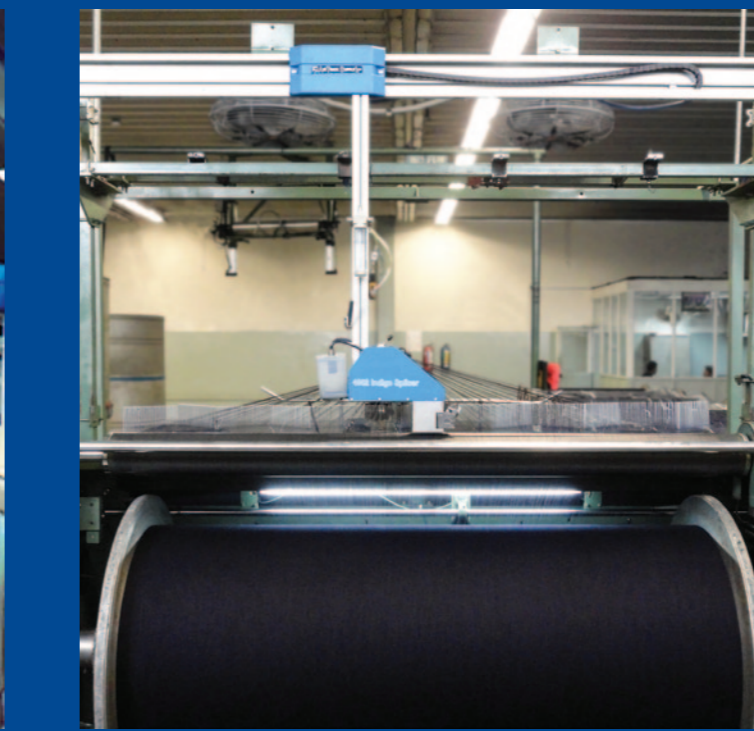
ATS "L" with INDIGO SPLICER 4662 installed on a Rebeamer - downstream of rope dyeing.
