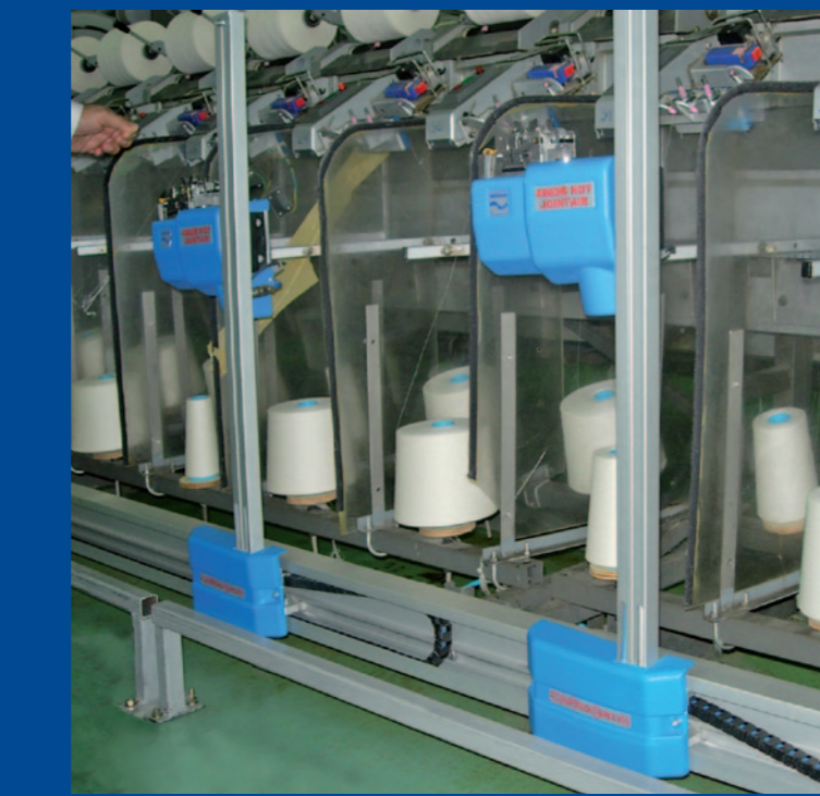
ATS "H" type with HOT JOINTAIR® 4983B installed from below on assembly winder .
