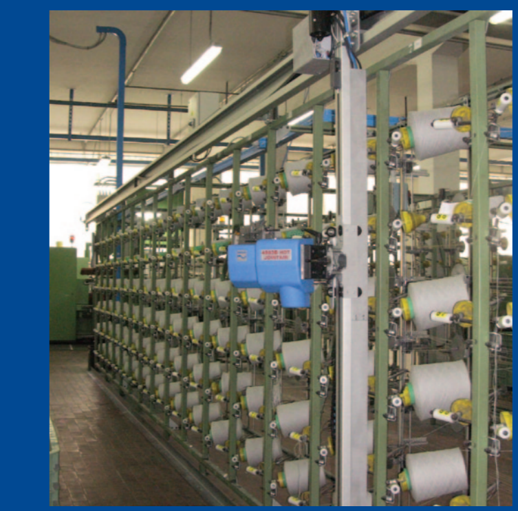
ATS "H" type with floor guide and HOT JOINTAIR® 4983B fitted on a slider for tail transfer at different level on sectional creel for wool warping.
