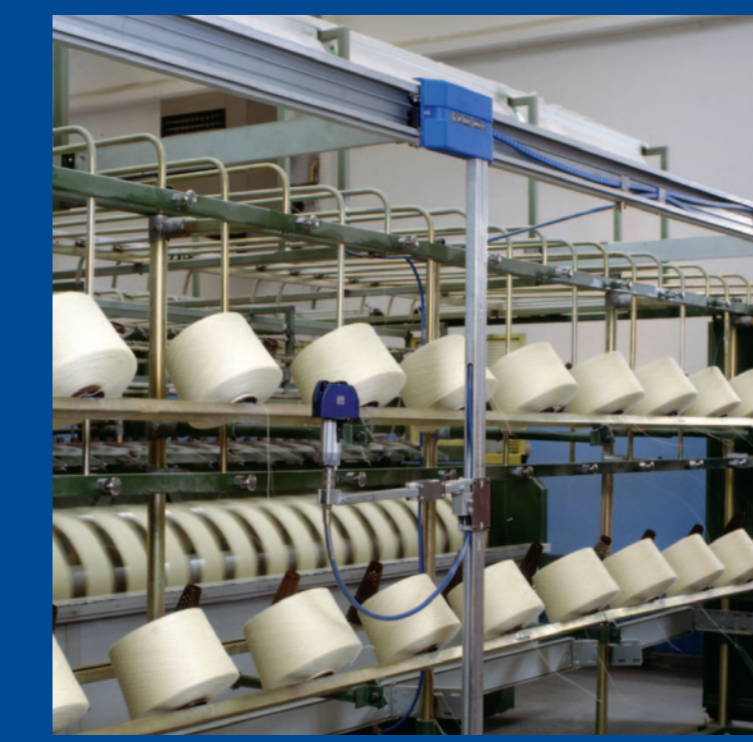
ATS "C" type with floor guide and JOINTAIR® 115 fitted on a slider to splice at different level worsted yarn on reeling machine creel.
