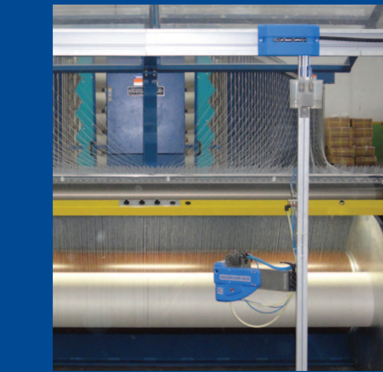
ATS "L" type with AQUASPLICER® 4923B placed in front of a fractional warping machine for cotton yarn.
