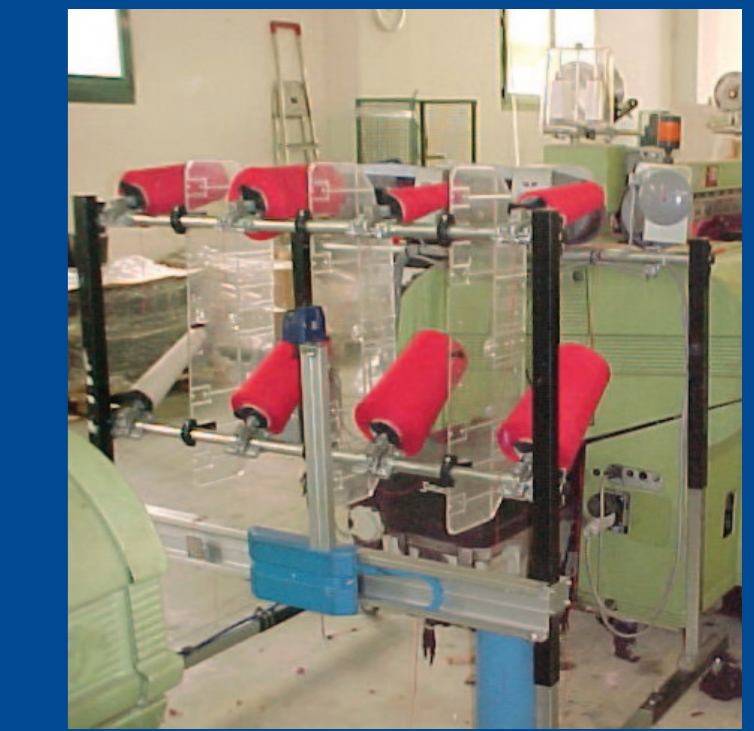
ATS "C" type with JOINTAIR® 115 fitted on weft creel for top-to tail join.
