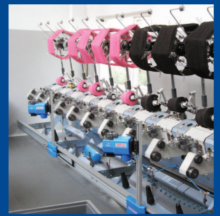
ATS "H" type with HOT JOINTAIR® 4984B on Hank to Cone winder processing worsted and wool yarns, cashmere and wool blends.
