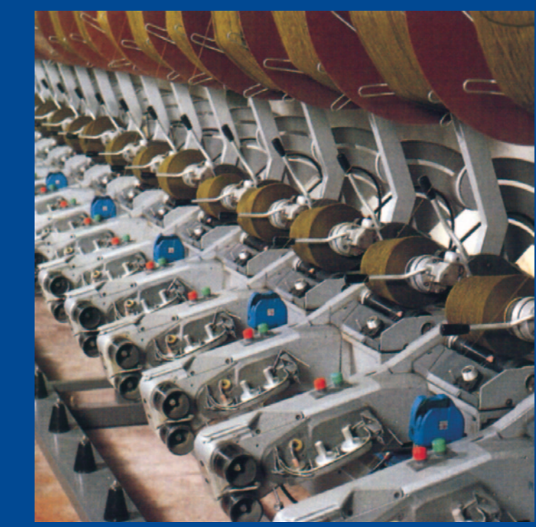
JOINTAIR® 115 fitted in a fixed position utilising one splicer for two winding heads on hank-to-cone winder processing wool/acrylic yarn.
