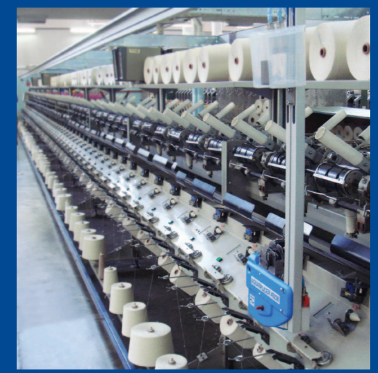
ATS "L" type with AQUASPLICER® 4923B installed on assembly winder equipped with moving blower.
